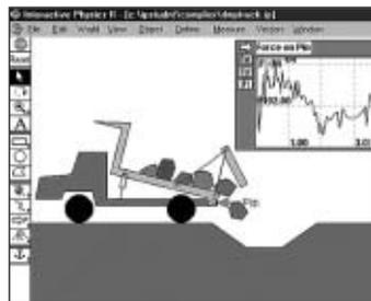
**Figure 1. Animation of the rolling, sliding and dumped stones in relation to the force to the pin**
